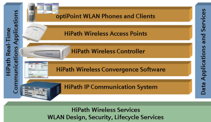
Figure 5. The Siemens HiPath Wireless Architecture
