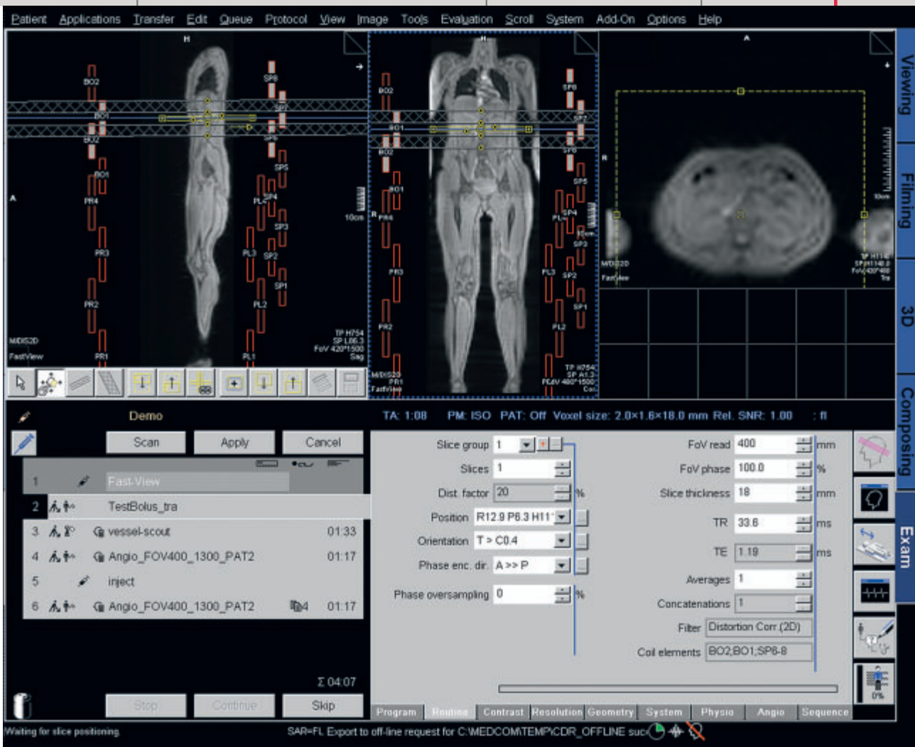
[ Figure 3 ] syngo TimCT FastView and planning of the TestBolus. The FastView sequence is based on a fast gradient echo sequence with fixed sequence parameters that runs without further sequence adjustments. The acquisition scan plane is transversal. Subsequent to data acquisition coronal and sagittal slices are automatically reformatted online. These reformats provide a gross overview of the patient's anatomy and serve as localizers to plan the transversal plane of the TestBolus sequence (yellow frame).
