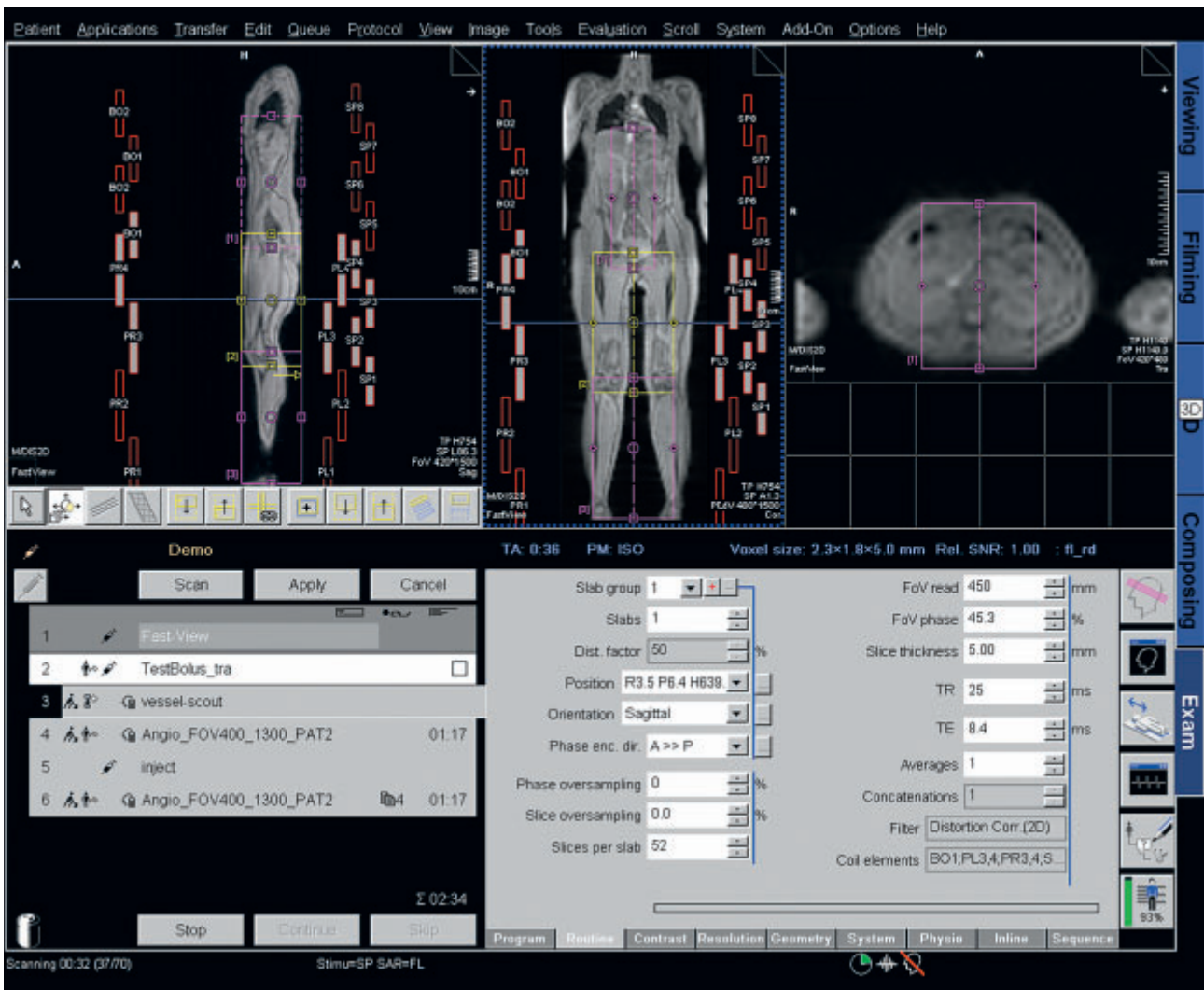
[ Figure 4 ] syngo TimCT FastView and planning of the VesselScout. Here the whole-body localizers provided by the FastView sequence serve as a basis to plan the VesselScout sequence. This is a multi-station rephased-dephased localizer in sagittal orientation with inline composing. The rephased-dephased sequence eliminates signal from static tissue and preserves signal from flowing blood thus providing a fast sagittal overview of the entire vessel tree.
