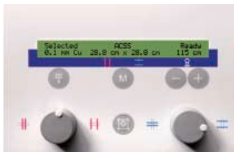
Convenient Cu filter selection on the collimator.
