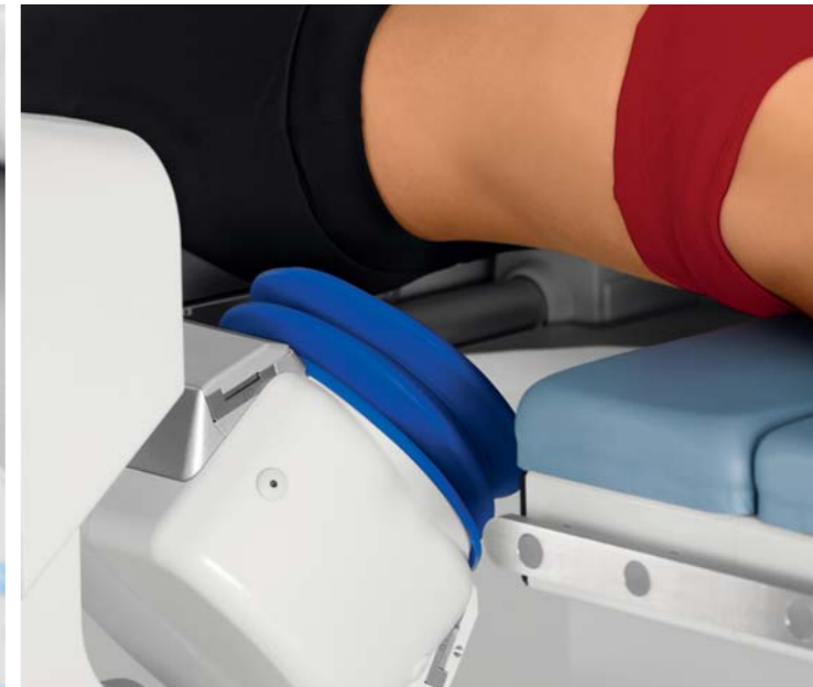
Motorized gel position – for contact-free pre-positioning of the patient and easy gel application.
