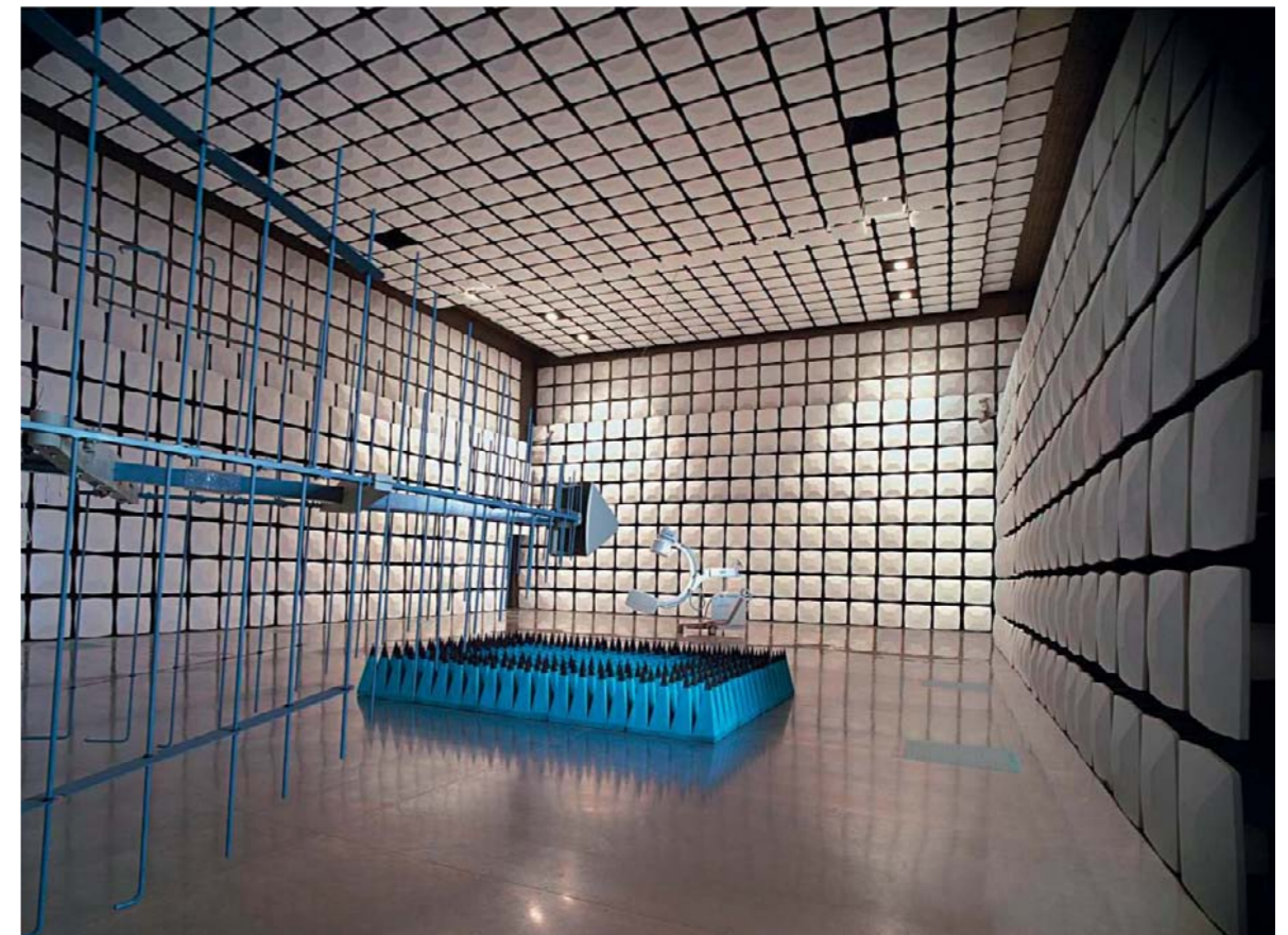
View into the absorber chamber which provides the electromagnetically "neutral" environment required for the product testing. With the shown testing facility the immunity against electromagnetic fields (e.g., broadcast, television, mobile radiocommunication etc.) can be tested.
