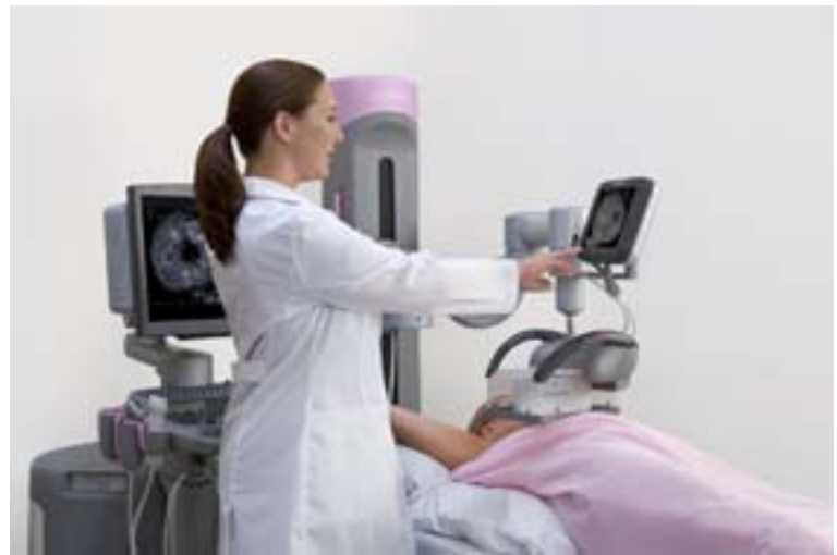
The ACUSON S2000™ Automated Breast Volume Scanner (ABVS) automatically acquires ultrasound volumes of the breast.
