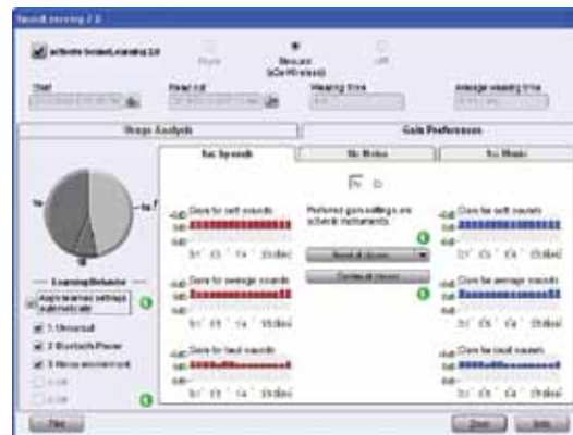
Figure 35: Gain Preferences tab in the SoundLearning 2.0 dialog. Learning has occurred for the Speech situation (1a), as indicated by the exclamation point (!). The HCP can then view the learned settings, and choose to either reset or apply them.
