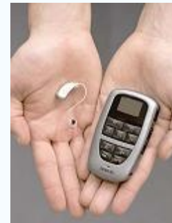
The Siemens Pure® 700 with the Siemens Tek® wireless enhancement is a Bluetooth® device that connects wirelessly to a phone. Photo courtesy of Siemens Hearing Instruments
