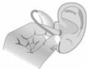
Fig. 6: Inserting the hearing instrument
