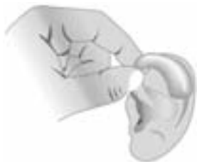
Fig. 7: Removing the hearing instrument
