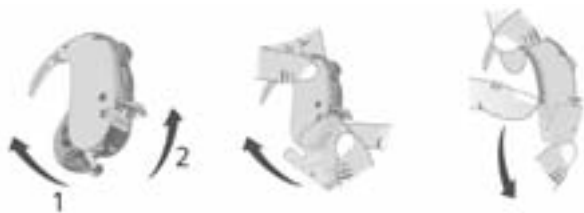
Fig. 10: Attaching the audio shoe
