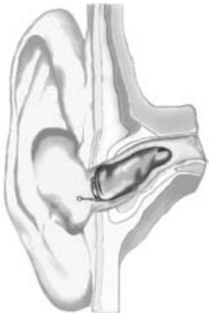
Fig. 5: Proper location of the Completely-in-the-Canal hearing instrument
