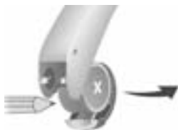
Fig. 4: Removing the battery
