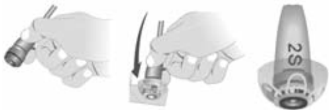
Fig. 9: Replacing the dome
