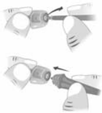
Fig. 10: Replacing the dome
