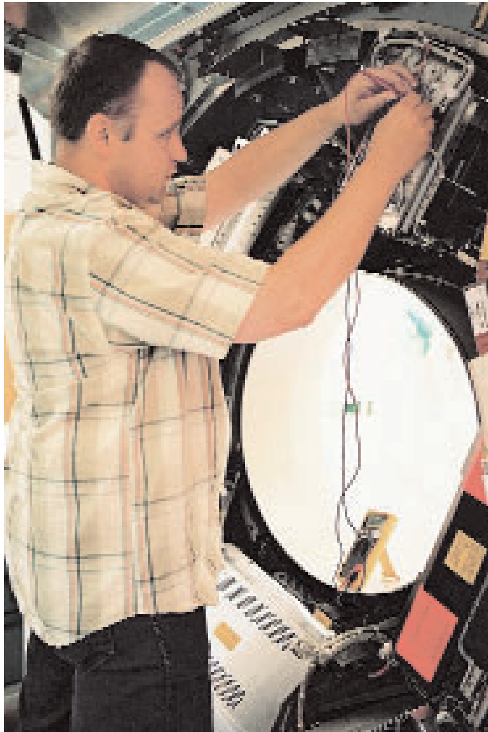
ASIDE FROM MAINTENANCE, engineers at UMC St. Radboud also perform repairs. Siemens trains them in the same courses they train their own service staff. Here, Ruud Engelen works on a SOMATOM® Sensation 64.
