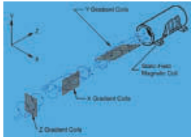
Figure 1. Typical gradient coil set used for localization of the MR signal. These coils are placed concentrically to each other within the magnet and are used sequentially for three-dimensional localization of the gradients to create images from the MR signal. Source: Jacobs MA, Ibrahim TS, Ouwerkerk R. MR Imaging: Brief Overview and Emerging Applications. Reprinted, with permission, from RadioGraphics . 2007; 27:1213–1229.
