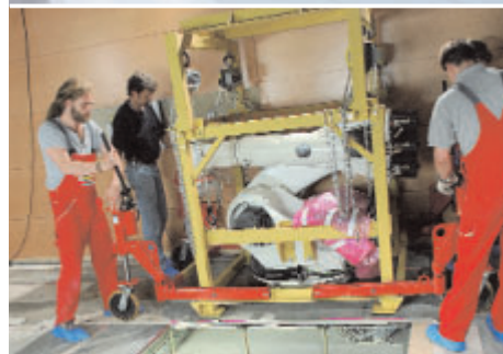
FROM THE LAB directly into the Heidelberg Ion Beam Therapy center: Thanks to the robot, patients can be positioned much more precisely for therapy. Top and center photos: test at Siemens; bottom photo: installation of the system at the customer site
