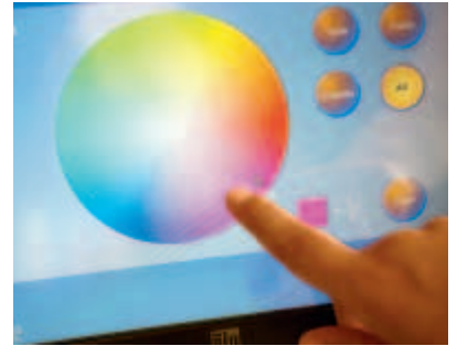
The user interface for Healthcare Lighting from Siemens Healthcare includes a touchscreen enabling convenient selection of colors from the entire color spectrum and many options to combine colors.
