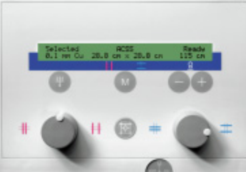
Cu filter selection displayed on the collimator.
