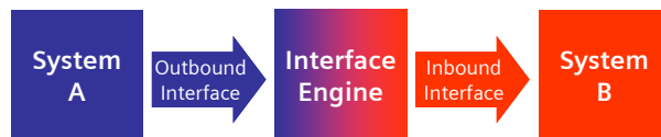
Figure 2. Data transformation via an interface engine Data leaving System A is reformatted by an interface engine so it can be forwarded and interpreted by System B.
