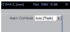
Figure 6 When selecting Matrix Coil Mode "Auto", the user interface indicates the Matrix Mode chosen by the system (in this example Triple Mode).
