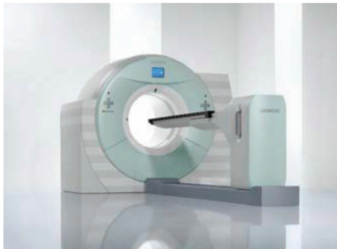
Figure 1. Siemens Biograph™ TruePoint™ and mCT, respectively, are leading-edge 3-dimensional (3D) lutetium oxyorthosilicate (LSO) high resolution and time-of-flight PET/CT devices, capable of simultaneous static, dynamic, and gated cardiovascular imaging through list mode (LM) acquisition. 9
