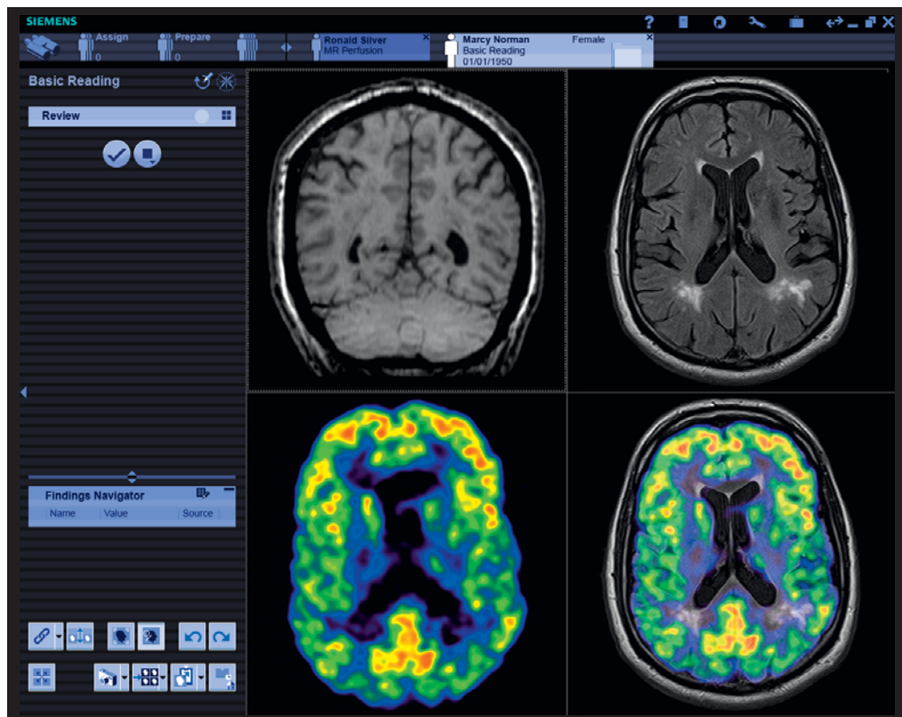
syngo Image Fusion. Enables you to view and “fuse” information from multiple modalities. In this example, PET data is subtly fused into a T2 Flair axial MR image (lower right).
