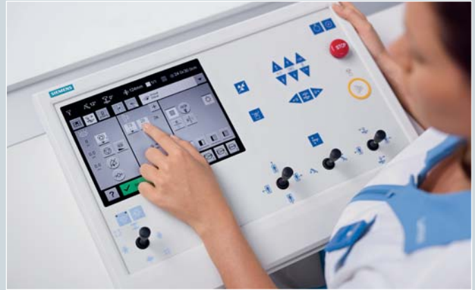
A real time saver: the newly designed intuitive and user-friendly remote control console with touch user interface.
